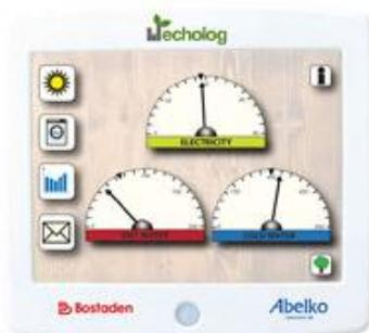
One of the interfaces has a main menu with "analog" meters showing consumption. The idea behind this "analog" representation is that the user recognizes this type of meter and finds it easier to understand. Current weather conditions are shown on the start page.
