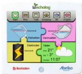
Another interface has symbolic graphics, whereby electricity consumption, for example, is shown in the form of a battery and hot water in the form of a teapot. This interface does not have a display in real time. The day's consumption is updated at a slower pace in order not to seem condemnatory when consumption is high at that time. The weather is shown on the start page too.
